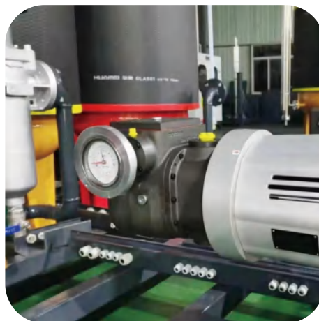
高压柱塞泵现场安装照片 Site installation photo of high-pressure plunger pump
