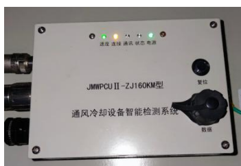
通风冷却设备智能监测系统 Intelligent Monitoring System For Ventilation And Cooling Equipment
